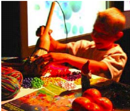
I/O Brush allows people to take attributes from objects in the physical world and immediately paint with them.
